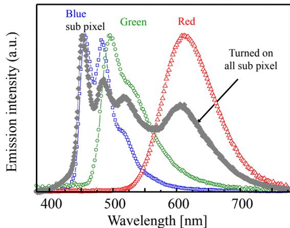
Fig. 4 Light spectra for RGB TOLED devices (components and full-stacked).
