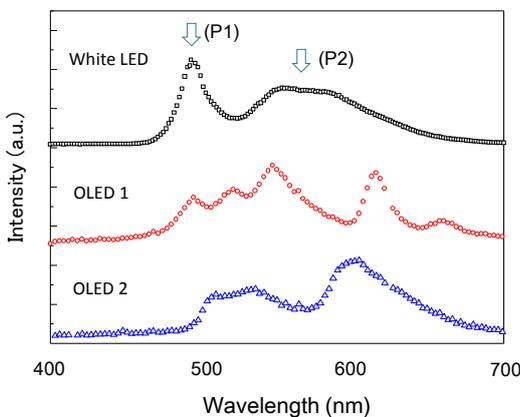
Fig. 8 Light spectra for the small dome (B) with white LEDs and two types of OLED lighting panels (OLED1 and OLED2).
