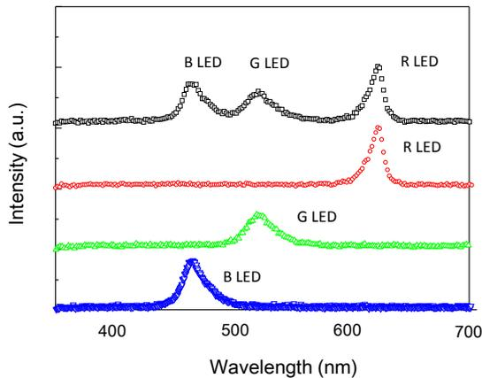
Fig. 7 (b) Light spectra for the small dome (A) with RGB inorganic LEDs.
