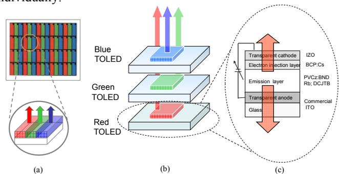
Fig. 1 Arrangement of RGB subpixels in a color display: (a) Conventional color display, (b) vertical stack type color display, (c) cross-sectional diagram of a red TOLED.
