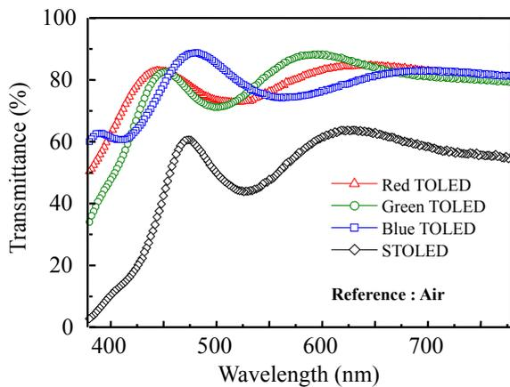
Fig. 3 Transmittance curves of R, G, and B devices, and of a full-stacked TOLED.
