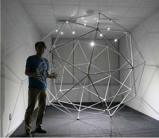
Fig. 2 The assembled lighting domes (A) and (B) (pentakis dodecahedrons).
