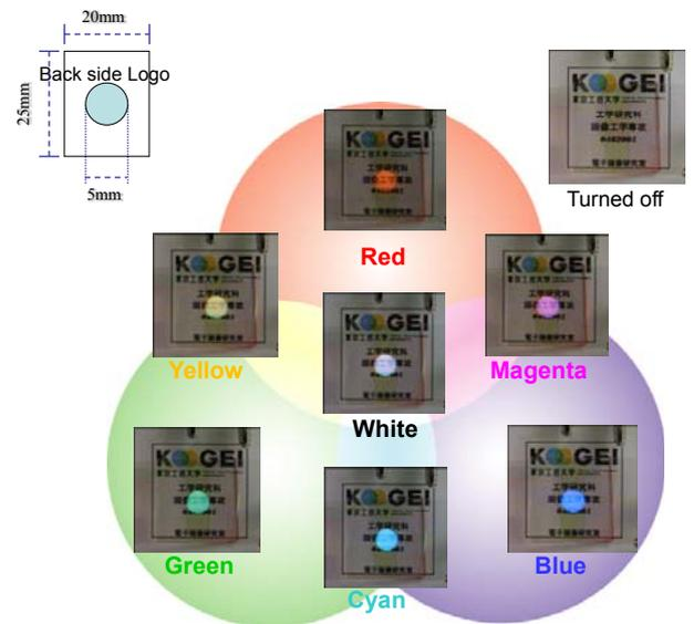
Fig. 6 The photographs of a stack-type transparent OLED (STOLED) show red, green, blue, cyan, magenta, yellow, and white colors.
