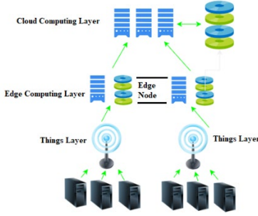
Fig. 1 Basic Edge Computing architecture
